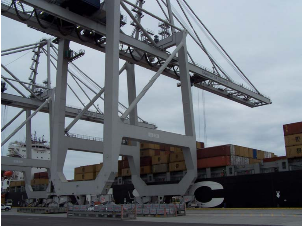
Panamax crane loading containers onto a cargo ship at the Garden City Terminal of the Port of Savannah
